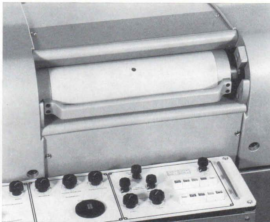
Daylight cassette and part of control panel.
